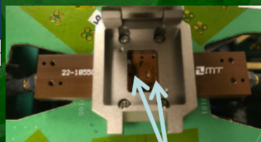
Dual Tx/Rx Patch antenna in contactor
